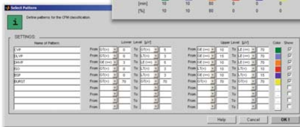
setup for automatic CFM segmentation: criteria for each class can be modified separately
