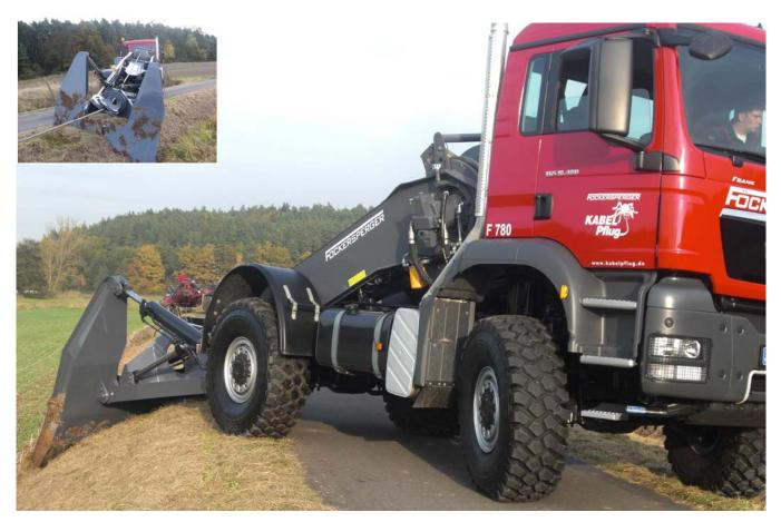
This winch vehicle has been highly developed down to the last detail, and stands out for short set-up times and rapid deployment from one site to another. The variable adjustment range of the long support arm, the tilting support shield and tipping winch all ensure perfect anchoring even on embankments, where the tractor vehicle stays on the road.
