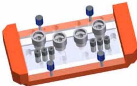
Figure 2 (above). A 3D-CAD design of the MOC including the support (red colour).
