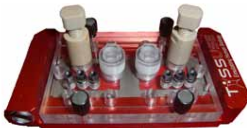
Figure 3 (below). A fully equipped MOC fixed in an autonomous support (red colour).
